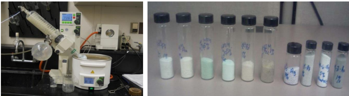
Figure 12 (a) Bench scale reactor system (b) Dried and calcinated photocatalysts
